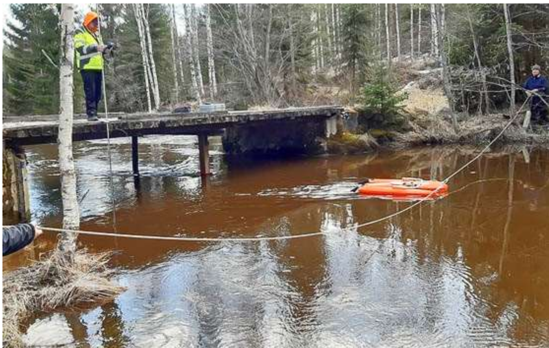
Figure 6. Discharge measurements performed by South-Eastern Finland ELY-centre and SYKE in the Rakkolanjoki (FIN) using an Acoustic Doppler Current Profiler (ADCP) and an electromagnetic flow meter. © Pekka Vähänäkki
